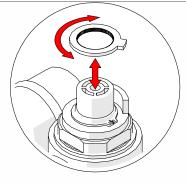
4. Remove both rings and turn tap spindle till desired temperature is achieved.
